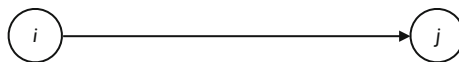
Fig. 2.6 The AoN representation of the technological link between activities i and j
